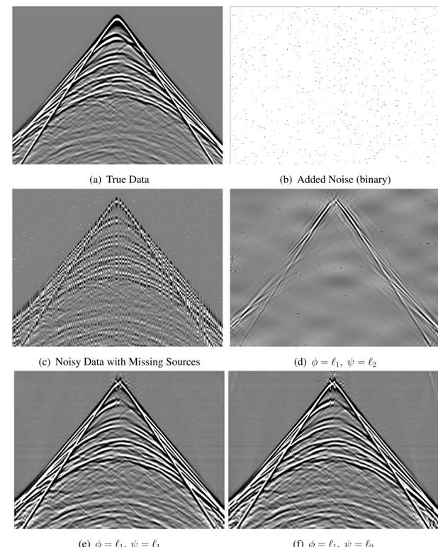
Figure 3: Interpolation and denoising results for BPDN in the curvelet domain. Observe the complete inaccuracy of smooth norms with large, sparse noise.
